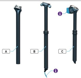
Bicycles ship with either a standard seatpost ( $\mathbf{A}$ ), mechanical dropper seatpost ( $\mathbf{B}$ ), or electronic dropper seatpost ( $\mathbf{C}$ ) installed. Identify the seatpost your model is equipped with, then follow the relevant instructions to adjust the seatpost height if required.
