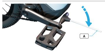
Using the corresponding hex key (A), inserted from the inside of the crank arm, tighten each pedal. When at the correct tension, the tool leaves a noticeable impression in the palm of your hand.
