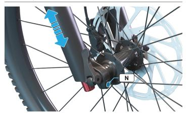
Cycle the fork, then using a hex key, gently tighten the pinch bolt (N), if your fork is pinch bolt equipped.
