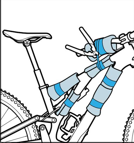
Remove the zip ties or rags securing the handlebar to the top tube.
